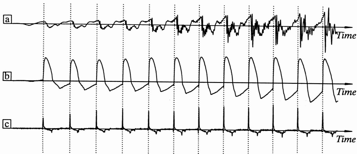
Fig. 14a-c. Speech signal (a), laryngogram (b), and differentiated laryngogram (c). The markers delimiting the individual periods were derived from the maxima of (c). Signal: transition [ja]; speaker WGH (male)
