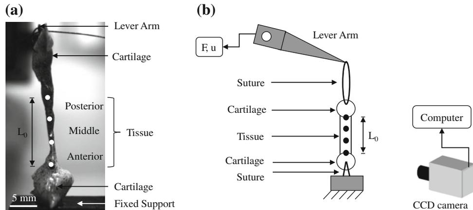
**FIGURE 1. The experimental setup for the cyclic tensile stretch test. (a) the vocal fold cover from a non-smoker (subject E). The four points that were optically tracked are shown as white circles. (b) Schematic drawing of the setup.**
