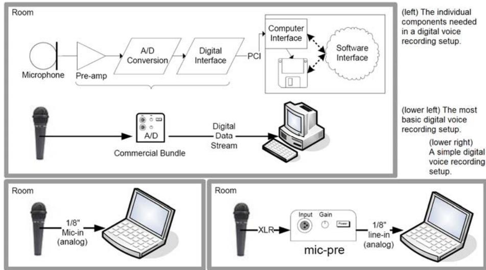
**Figure 1.** A digital voice recording setup requires a microphone, microphone preamplifier, analog-to-digital converter, digital interface, software interface, and recording environment. Many of these components are often bundled together.
