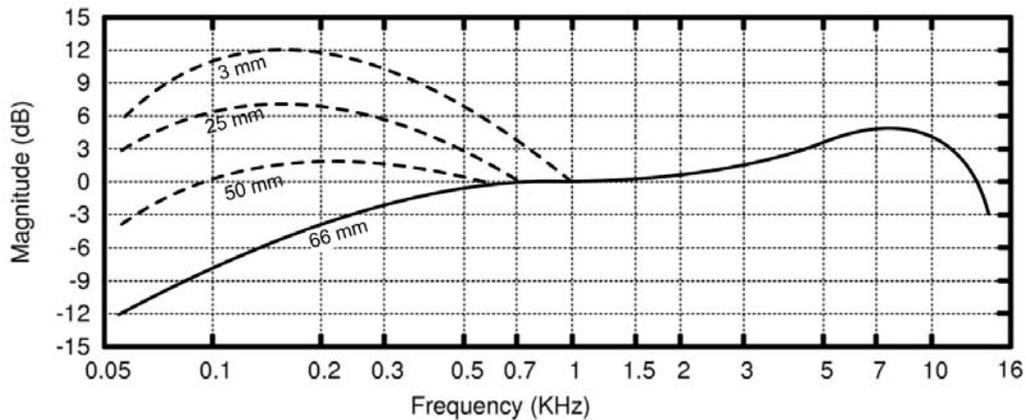
**Figure 3.** (solid line) *Frequency Response*: The sensitivity of a component to various frequencies (i.e., the amount in dB each frequency is amplified or attenuated where 0 dB means no change), usually graphed as an amplitude or gain (vertical axis) plotted against frequency (horizontal axis). (dashed lines) *Proximity Effect*: For directional microphones, the frequency response of the microphone changes at the low frequency end, as the microphone-to-mouth distance changes.
