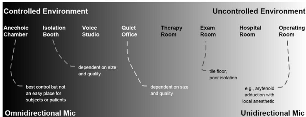
**Figure 4.** An example of various rooms where voice signals are recorded, illustrating the range from the most controlled to the most uncontrolled acoustic environment with preferred microphone type.
